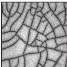
The spider-web pattern of cracking is different from a break in the aspect that it cannot be felt on the surface, unless using a fingernail; however, it does become more visually apparent when the surface is dusty or magnified. While these may appear as imperfections, crazing does not affect the performance or life span of your ceramic charcoal barbecue; therefore, not a warranty issue. The process of crazing effectively increases the toughness of the unit.
